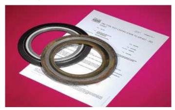
**Composition:** 316L stainless steel inner support ring, winding strip with PTFE inner seal, graphite outer seal and carbon steel outer ring material on standard design.
